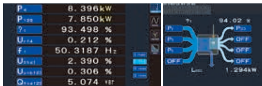
P4: DC power (panel output) f1: Frequency P123: 3-phase power (power conditioner output) Urf4: Ripple rate Uthd1: Voltage total harmonic distortion η1: Conversion efficiency Uunb123: Unbalance rate Qfnd123: Fundamental wave reactive power
